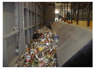
Steel cans are moving along a conveyor belt on their way up to the sorting room for processing. After the cans are sorted they will be stored in a bin under the sort line until they are fed on the baler feed conveyor and baled into bales weighing around 1800 lbs.
